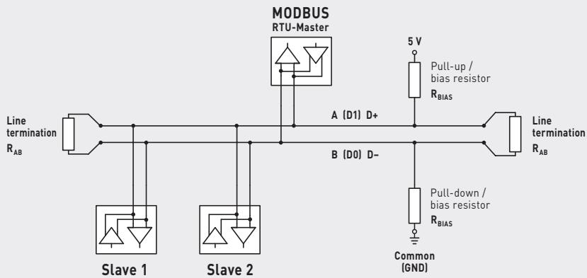
The bus termination can be fully switched on or off via DIP switches. In doing so, both the BIAS resistors, which can be activated separately via DIP 2, and the line termination resistor between the two data lines A and B are switched on or off.
